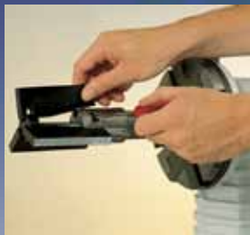
Fast adjustment of the pipe dimension
