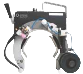
ORBIWELD TP 600 with KD 3-100 cold wire feed
